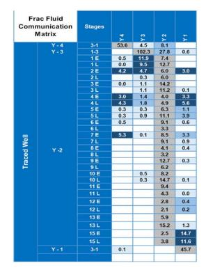
Figure 28—Communication matrix for pad Y
