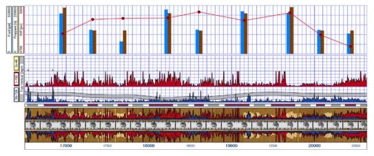
Figure 9—Spectral gamma ray log for TF-1H Well
